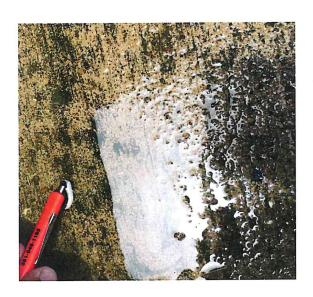
Subject: Demonstration of magnetic property of the accumulated metallic particles on Citizen 43's front sidewalk after power washing the exterior front alcove and front sidewalk twice
