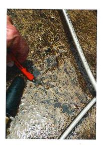
Subject: Demonstration of magnetic property of the accumulated metallic particles power washed from Citizen 43's front sidewalk
