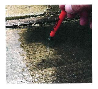
Subject: Demonstration of magnetic property of the accumulated metallic particles power washed from Citizen 43's front sidewalk
