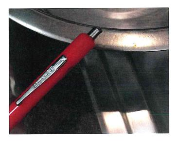
Subject: Demonstration of magnetic property of the metallic particles accumulated in the dog bowl (stainless steel) within ~12 hours (6 am-6
