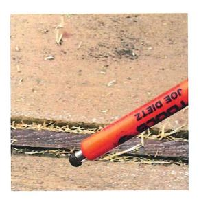
Subject: Demonstration of magnetic property of the accumulated metallic particles power washed from Citizen 43's front sidewalk
