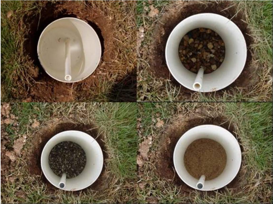
**Figure 3. 10 The installation of supporting layers within a sampler (lysimeter)**
