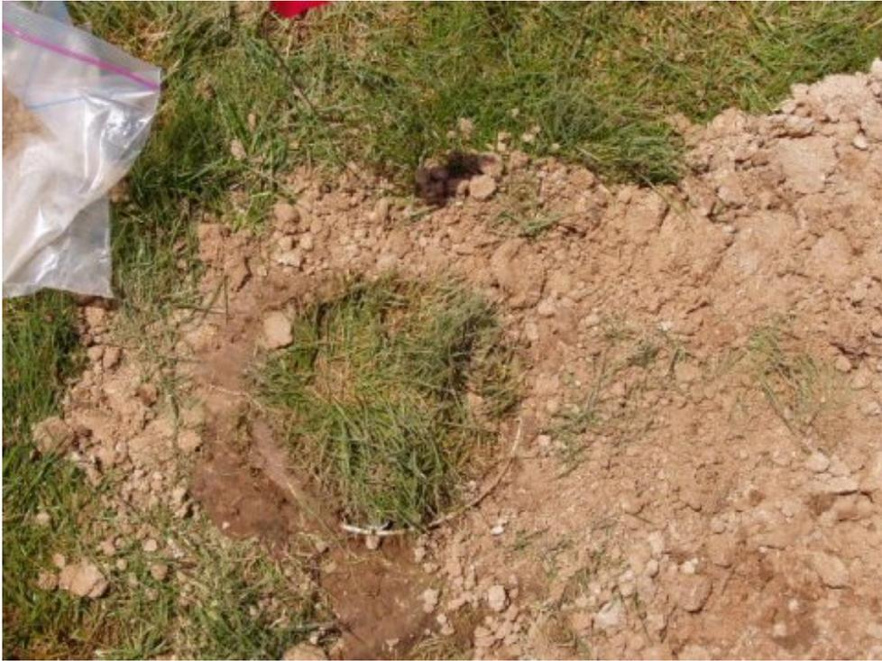
**Figure 3. 11 Right after installation of a sampler into ground**
