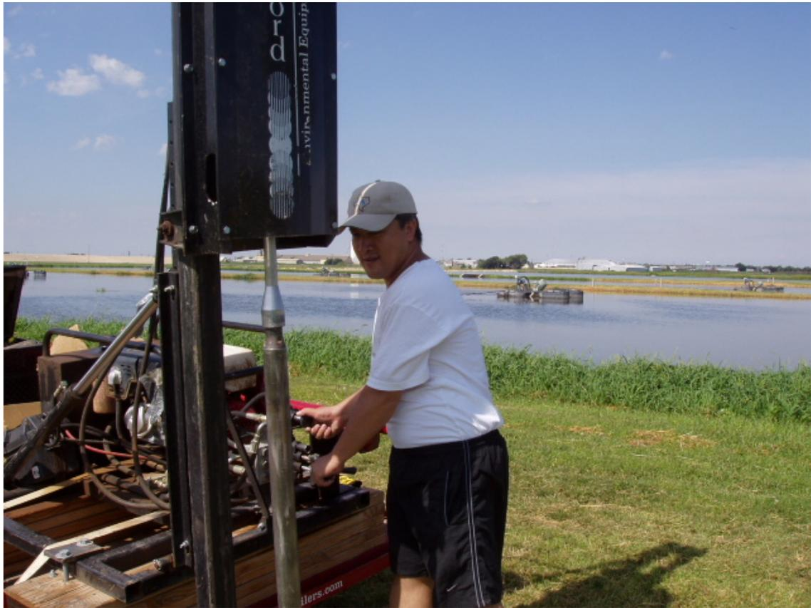
**Figure 3. 13 Deep soil sampling in process**
