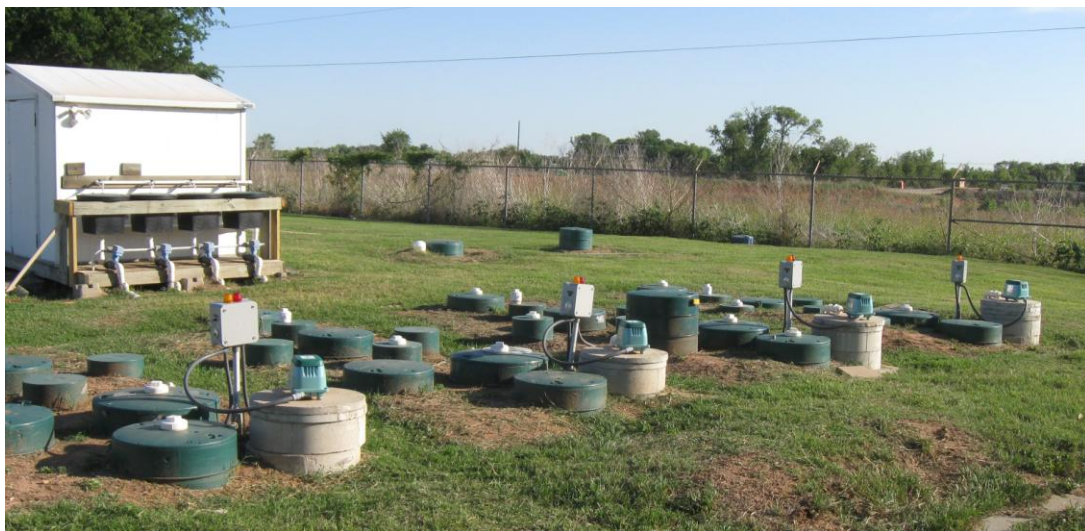
Figure 2. The enlarged new configuration showing the 4 aerobic systems with standard control panels and blowers in the foreground and the new, larger-capacity dosing buckets re-plumbed at the dosing shed in the background.
