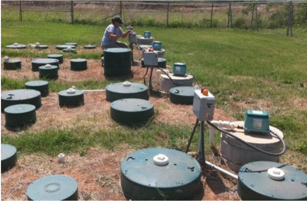
Figure 1. Graduate student, Amy Price, setting up control panels for the aerobic systems.
