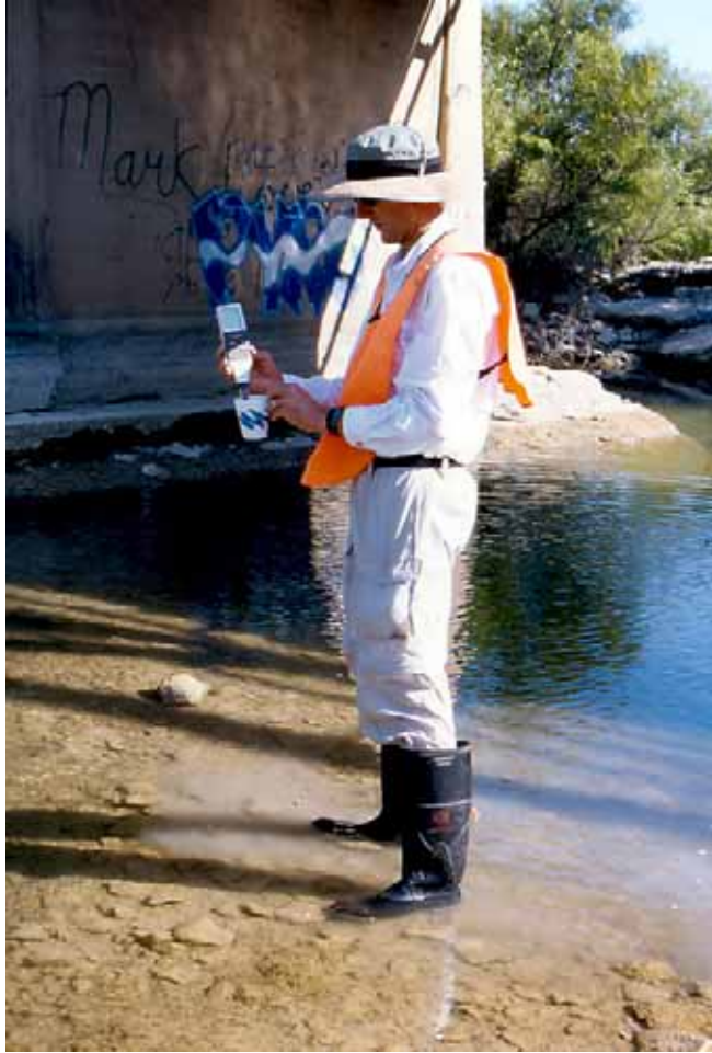
Figure 4. Measuring water temperature, conductivity, and total dissolved solids (TDS) concentration on Mustang Creek using a Corning Checkmate 90 probe.
