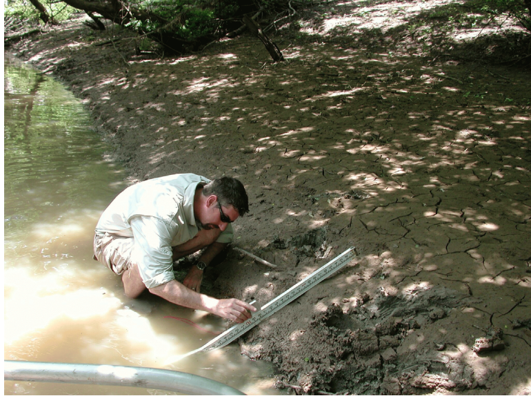
Measuring a Bank Angle with a Clinometer and Range Pole
