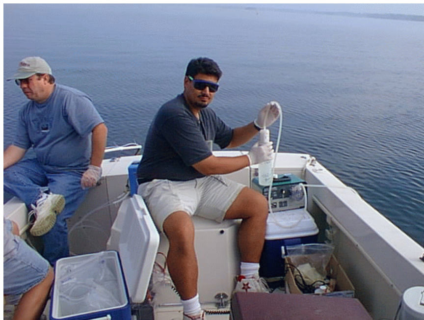
Collecting a Dissolved Metals Sample with a Cartridge Filter and Peristaltic Pump
