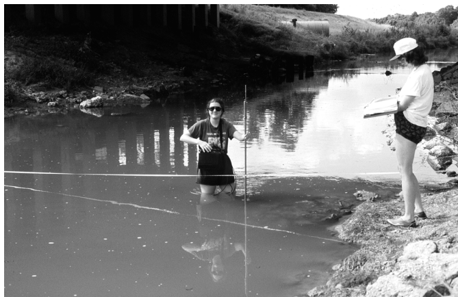
Making a Flow Measurement with an Electronic Meter
