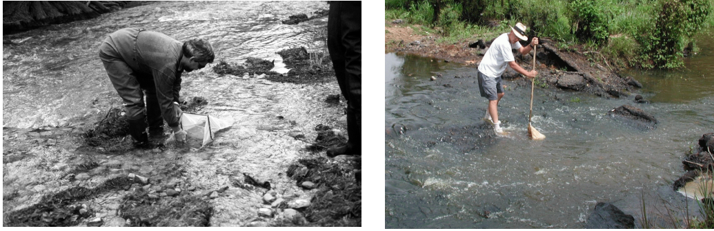
Collecting Benthic Macroinvertebrates with a Surber Sampler (left) and a Kick Net (right)
