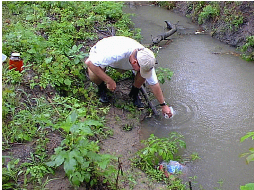
Collecting a Routine Water Sample From a Small Stream by Immersing the Container
