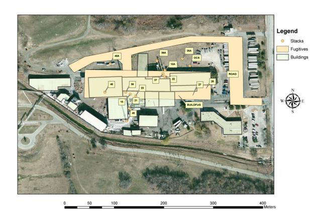
Figure 3-4: Graphical Representation of Modeled Emission Source Locations and Building Configuration
