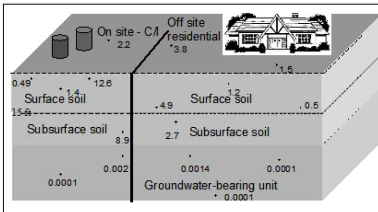
**Figure 6. Sampling points and COC X concentrations (mg/kg and mg/L).**
