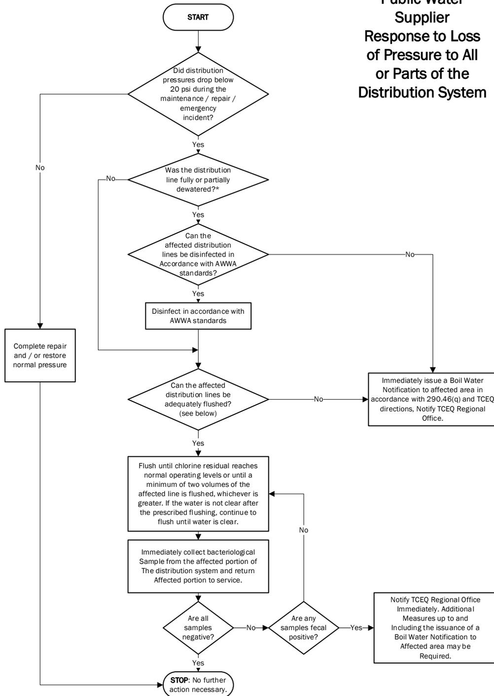
**The following directions are outlined in a flowchart on p. 129 and cover special precautions for public water supplier response to loss of pressure to all or parts of the distribution system. [30 TAC 290.47(e)]**
