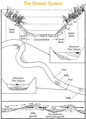
The above diagram shows the water flow and major structures of a stream. Notice how the pools and riffles alternate. A major feature of the riffle is that water flows through the gravel as well as over it. This enables small fish and small benthic invertebrates to obtain the oxygen they need while being protected from predation by larger organisms such as fish. Source: Kentucky Division of Water
