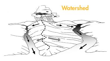
Watersheds are also commonly called *drainage basins* or *drainage areas*. The total area of land that contributes stormwater to the outlet is determined by topographic boundaries. A ridge or other area of elevated land (called a *divide*) separates one watershed from another. A stream on one side of the divide will flow to a different outlet than one that is on the other side of the divide.
