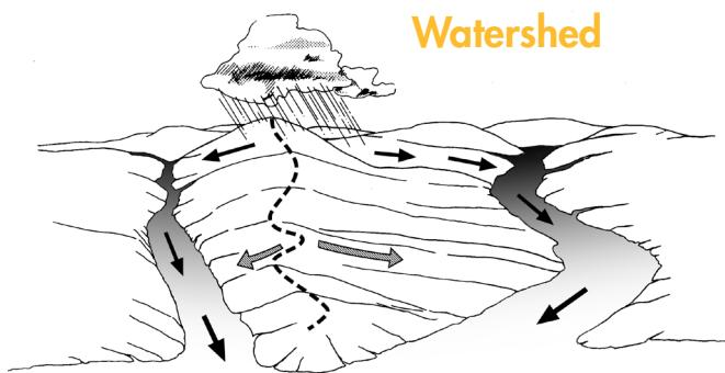
Watersheds are also commonly called *drainage basins* or *drainage areas*. The total area of land that contributes stormwater to the outlet is determined by topographic boundaries. A ridge or other area of elevated land (called a *divide*) separates one watershed from another. A stream on one side of the divide will flow to a different outlet than one that is on the other side of the divide.
