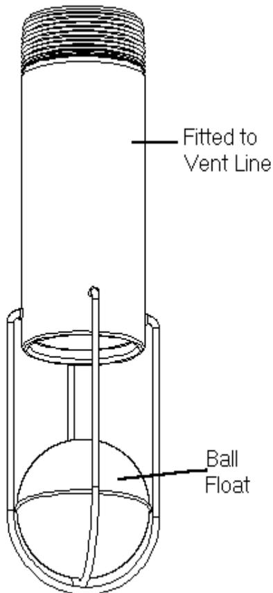
Figure 5. The ball float valve with the ball at the bottom of the cage and the vent line open. The product is below the cage.
