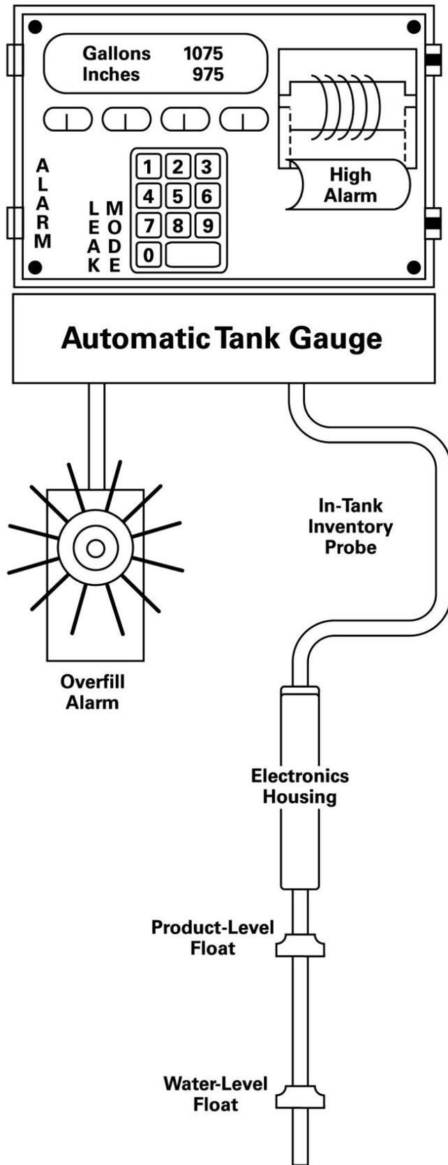
Figure 7. Overfill alarm.
