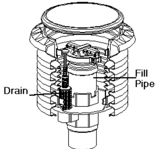
Figure 2. Spill bucket with a drain valve.
