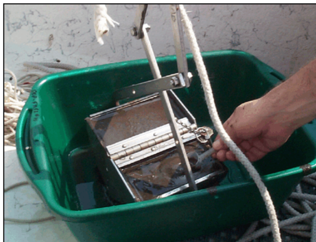
Figure 6.6. Collecting a sample directly from the dredge.
