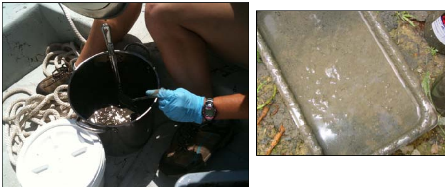
Figure 6.5. Compositing a sediment sample in a bucket or pan.
