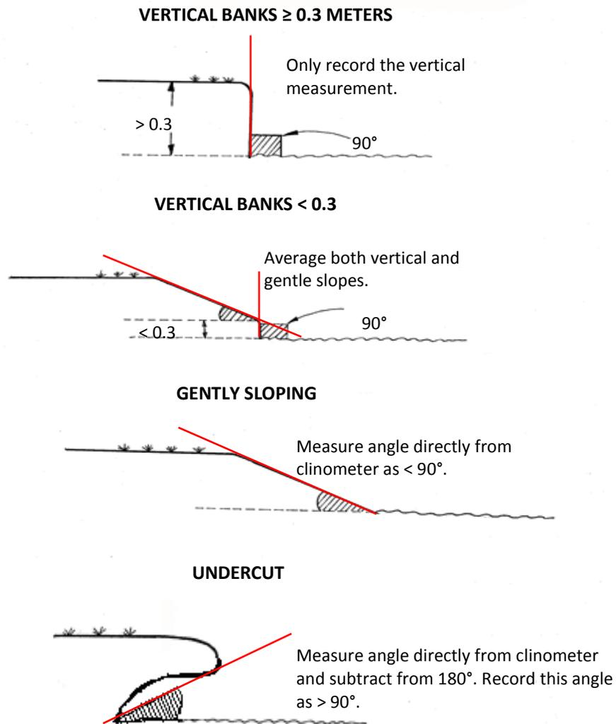
**Figure 9.6.** Bank-angle measurements.
