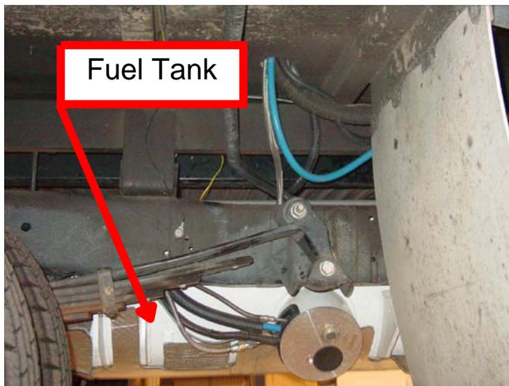
The fuel fill system is made up of the following items: 3/8 remote fill line-nozzle to filter, 3/8 remote fill line-filter to tank, fuel filter assembly, fuel filter bracket, fill valve, custom fill valve bracket, bolt and washer (M5 x 16), bolt for the filter bracket mounting (M8 x 1.25 x 20), and a wormgear clamp. Figure 10 below shows dual fill valves installed in FL01. The second fill valve was installed to fill the auxiliary tank used for development purposes.
