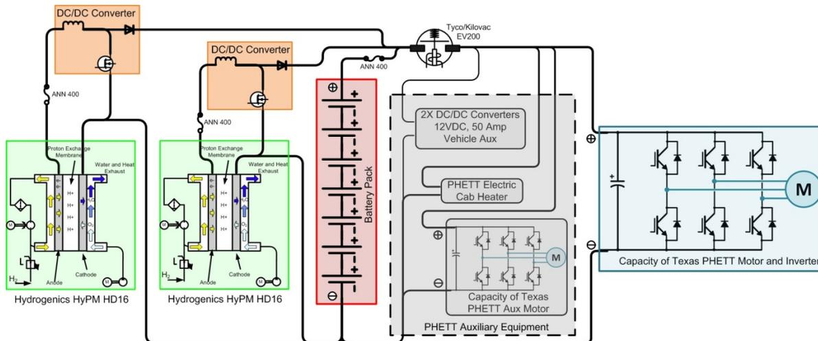
**Figure 1: Fuel cell architecture with two fuel cells operating in parallel**
