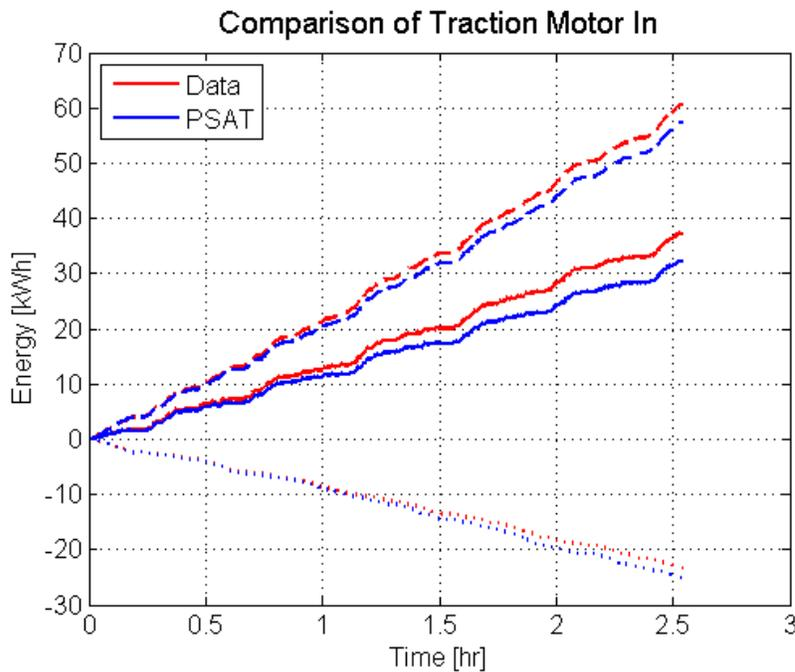
Figure 8: Comparison of traction motor energy for data on March 8, 2013, versus the PSAT model. Solid lines show overall energy use, while dashed lines show energy to the wheels and the dotted lines show regenerative braking energy.
