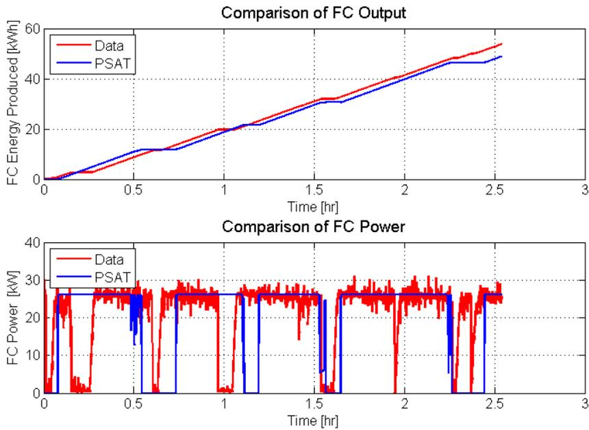
Figure 6: Comparison of fuel cell output power and energy produced for data on March 8, 2013, versus the PSAT model.
