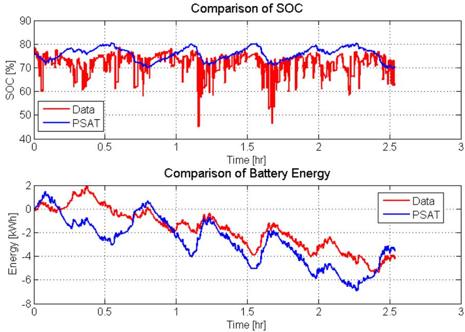
Figure 7: Comparison of battery performance for data on March 8, 2013, versus the PSAT model.
