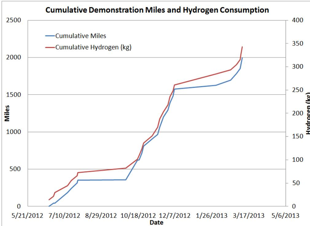
**Figure 4: Mileage and hydrogen consumption during the demonstration.**
