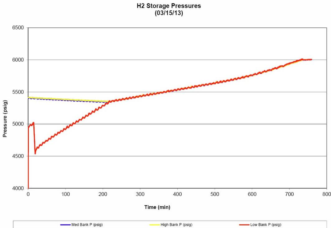
**Figure 9: Hydrogen storage pressures during hydrogen production.**
