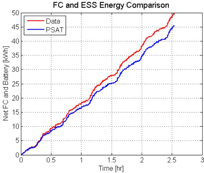
Figure 5: Comparison of overall energy consumption for data on March 8, 2013, versus the PSAT model.
