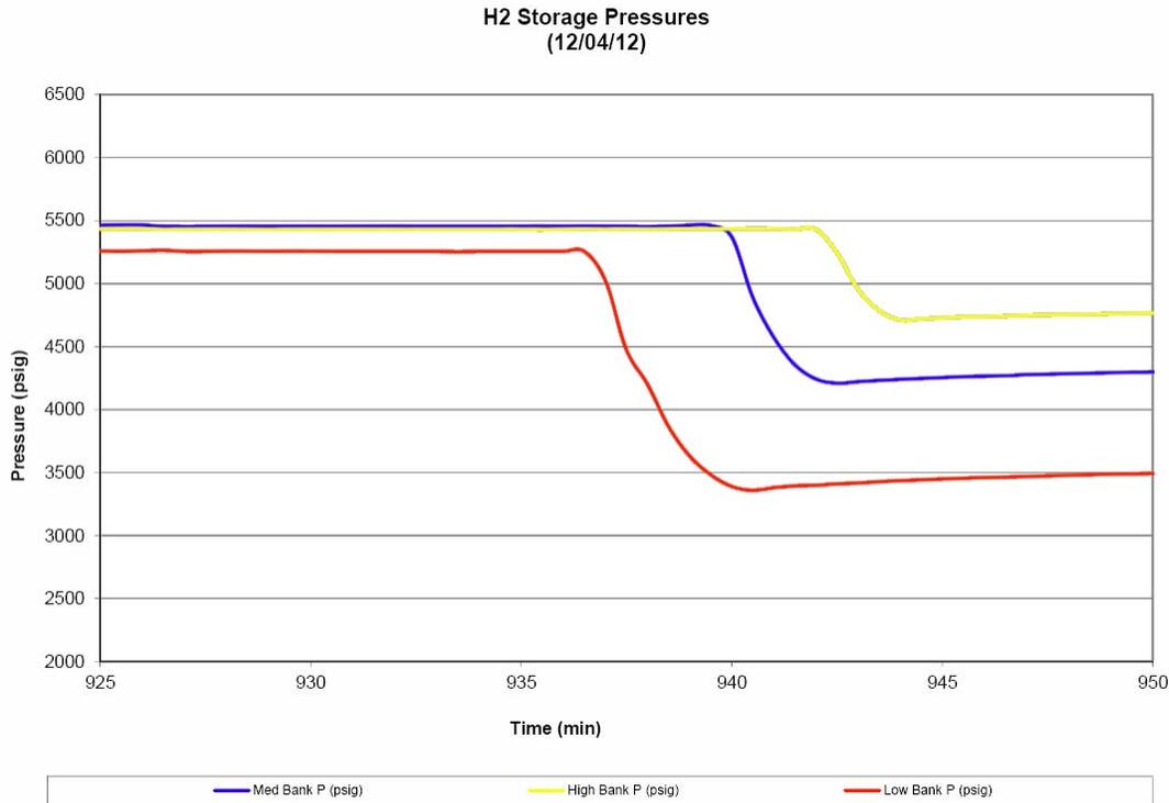
**Figure 10: Hydrogen storage pressures during bus refueling.**
