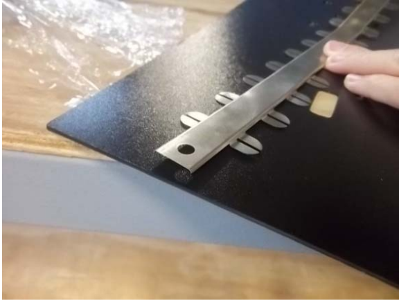
Figure 1. prototype bus bar fabricated using annealed non-hardened material
