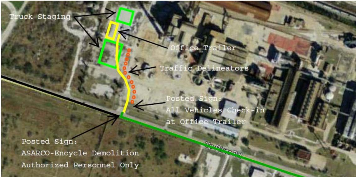
Figure 5 - Traffic Control to Navigation Blvd.
