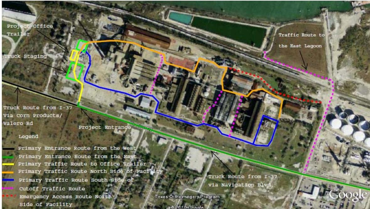
Figure 3 – Plan View of Facility Traffic Routes
