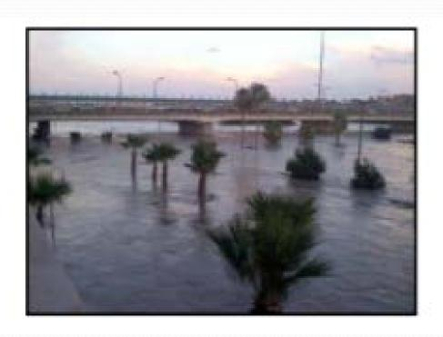
Flood flow is reported as a flow severity of 4. Flood flows are those that leave the confines of the normal stream channel and move out onto the floodplain (either side of the stream)
