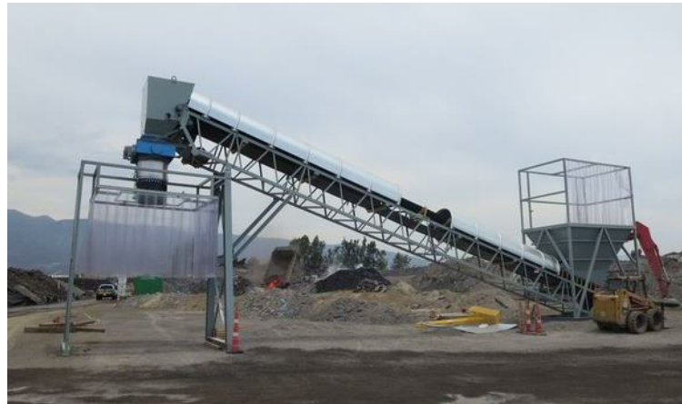
Figure 5.3.1 – Possible Solution for Truck-Loading Station
