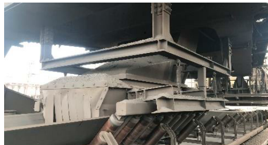
Figure 4.4.5.2 – RCL01 Lower Material Transfer
