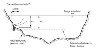
b) Example: Unbounded Cross - Section Looking Downstream (Small Buoyant Jet Discharge Into Large Lake or Reservoir)
