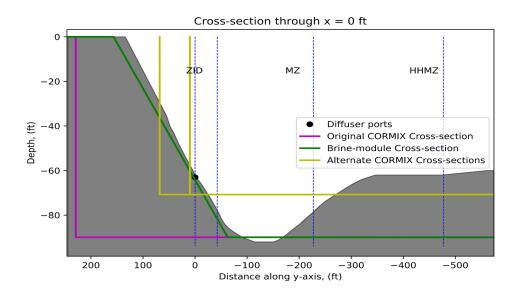
The vertical line at 0 along the bottom of the figure is the location of the outfall with relationship to the bank at the latitude and longitude. It is shown at 65 feet by the dot on the green dotted line. The vertical and horizontal purple lines show the ED and Port's
