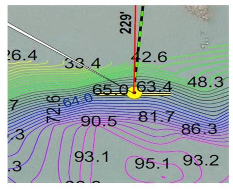
And what is also very obvious from this figure is that the plume for most of the tidal cycle never gets over the 90-foot hole. The majority of the time, the plume turns in or out with the channel current, only going a few feet from ports before turning. The Port argues that the effluent is then carried with the current, which would not be into the 90-foot hole.
