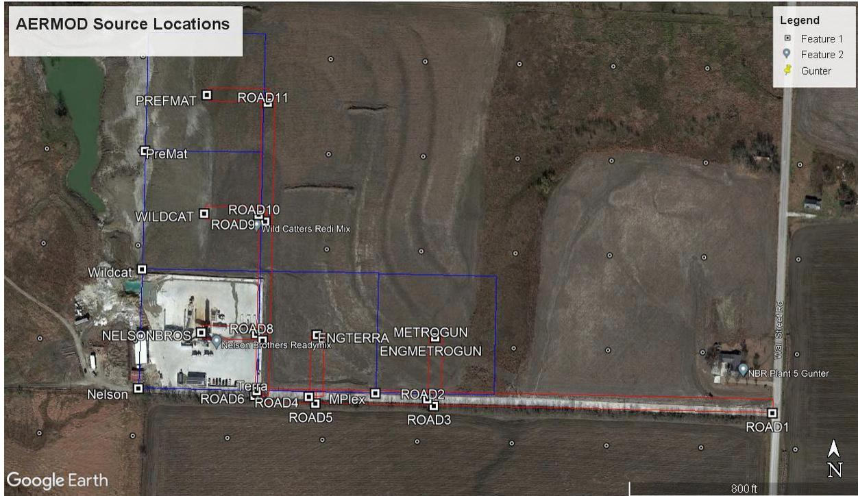
For AERMOD, the truck traffic fugitive dust was modeled using current US Environmental Protection Agency (EPA) recommendations for haul road truck traffic<sup>5</sup>. The “area source” approach listed by EPA was followed. The road width was assumed to be 8.0 meters, which would represent a standard two-lane roadway and the truck height from the specification data described earlier was 12 feet.
