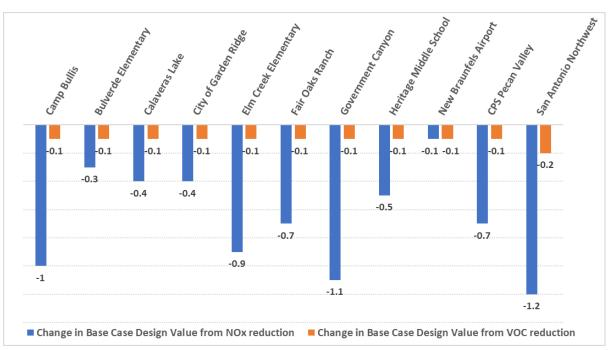
Figure 5-13: Modeled Impact of NO<sub>x</sub> and VOC Reductions on 2019 Ozone DVB
