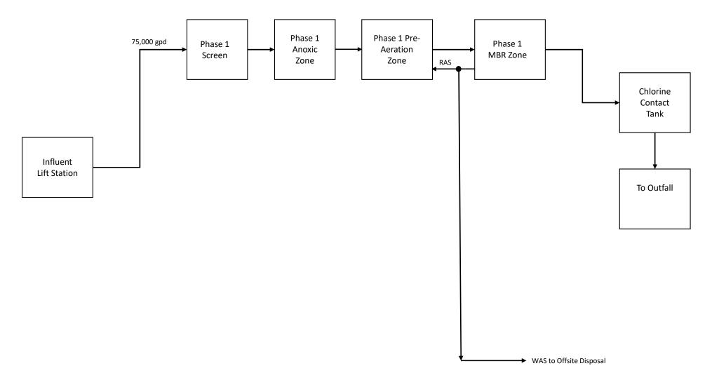
Attachment 8 – Process Flow Diagram Phase 2
