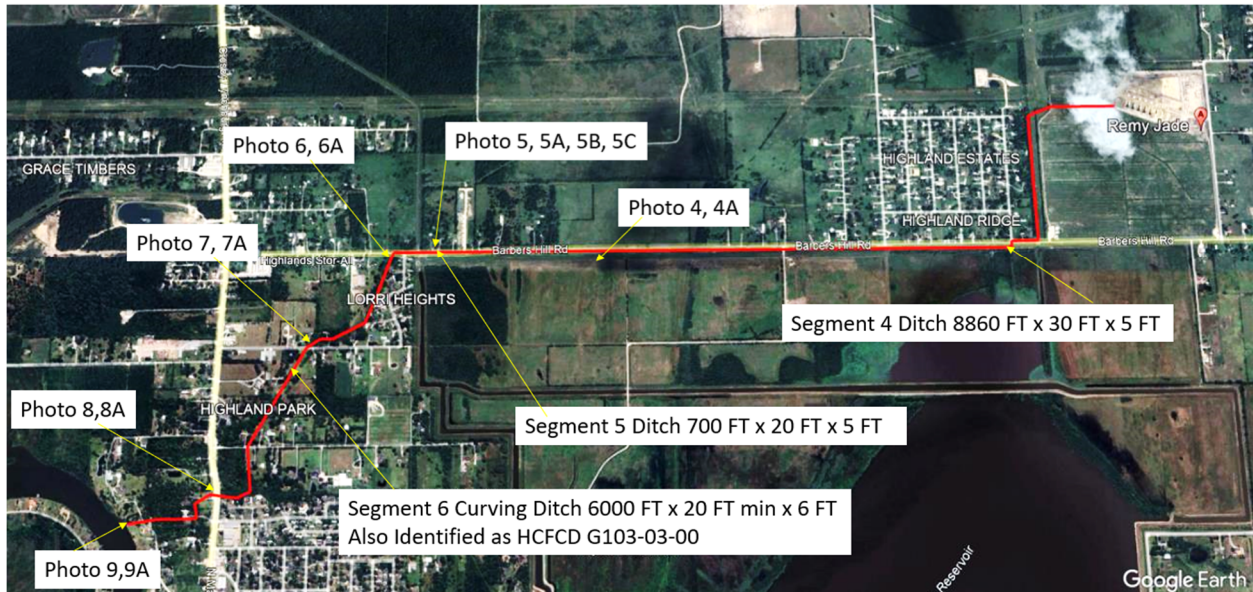
Figure 3 Flow Path for Remy Jade Power Plant from Barbers Hill Road to Outlet to San Jacinto River Segment 1001 and Photograph Locations
