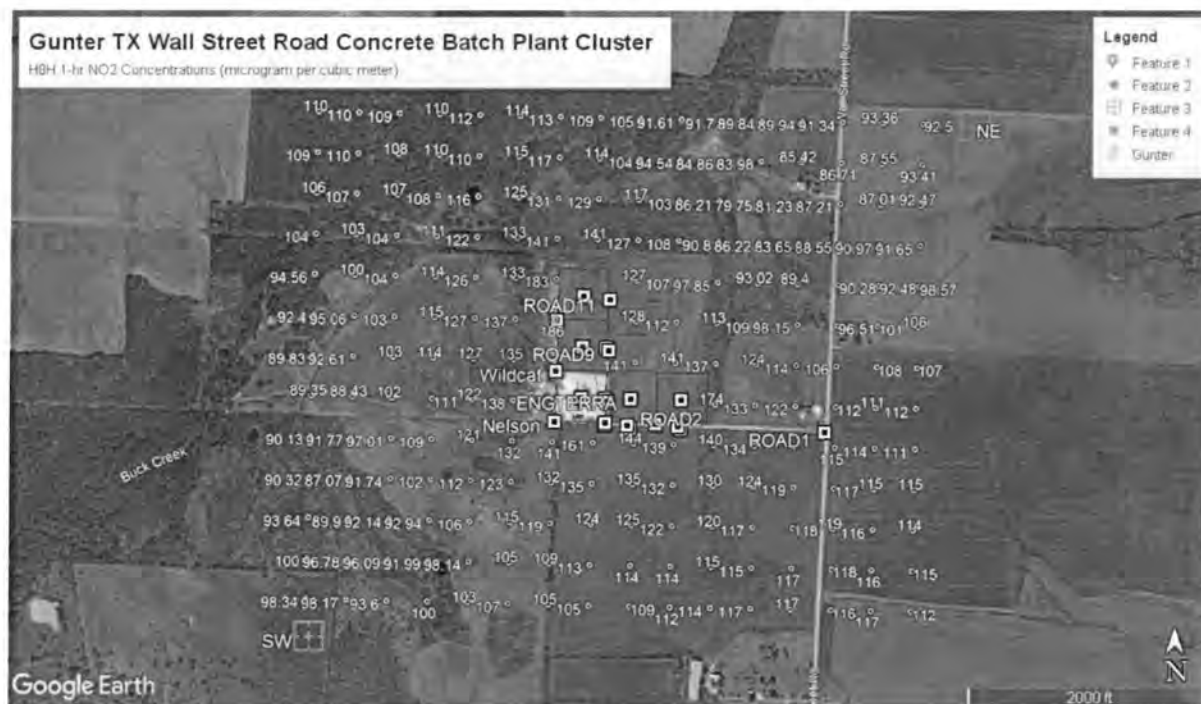
Figure 5 Wall Street Road Concrete Batch Plant Cluster H8H 1-hour NO 2 Concentrations (µg/m 3 )
