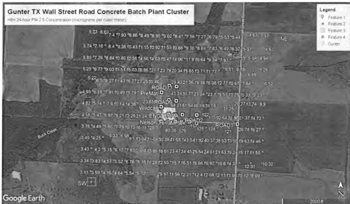
Figure 4 Wall Street Road Concrete Batch Plant Cluster H8H 24-hour PM 10 Concentrations (µg/m 3 )
