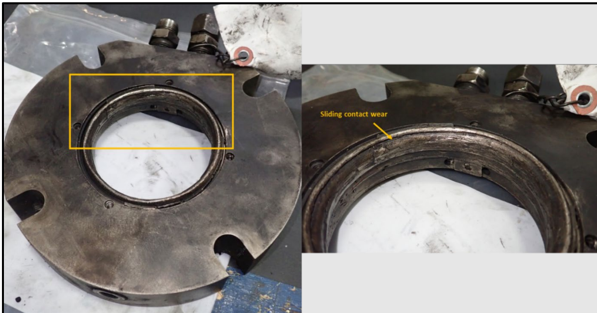
Figure 24. Smeared metal on inside surface of seal gland that indicates sliding contact with the pump shaft. (Credit: Stress Engineering)
