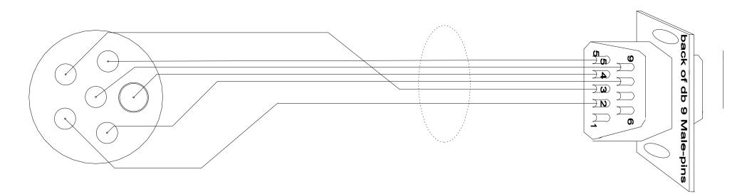
Cut 9 to 9 pin cable Brown Pin 2 to zeno RXD Red Pin 3 to zeno TXD Yellow Pin 5 to GND Orange Pin 4 to 10-16 Vdc Violent Pin 8 to Comm 2 A (SDi-12) White Pin 9 to ???
