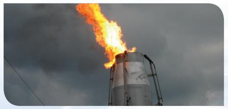
This is an example of an air-assisted flare effectively burning and destroying waste gas (achieving high efficiency). Notice the flame.
