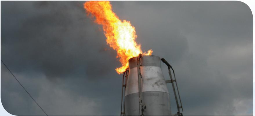
*This is an example of an air-assisted flare effectively burning and destroying waste gas (achieving high efficiency). Notice the flame.*
