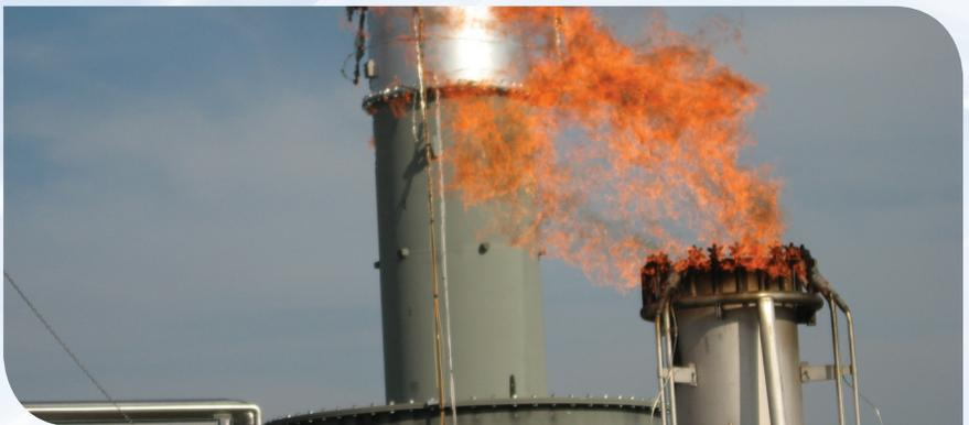
*This is an example of a steam-assisted flare effectively burning and destroying waste gas (achieving high efficiency). Notice the flame.
