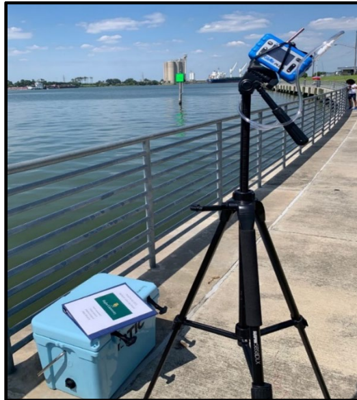
Figure 2: Markes single pump system to sample sorbent tubes (September 2021) at the San Jacinto Battleground Historic Site
