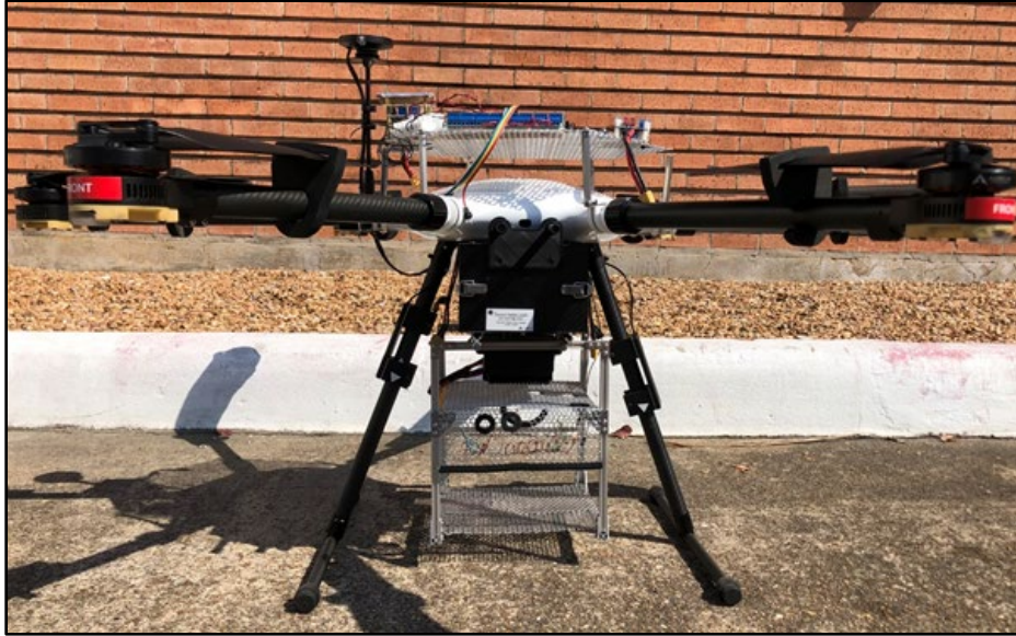
Figure 63: Chassis mounted to the bottom of the drone.
