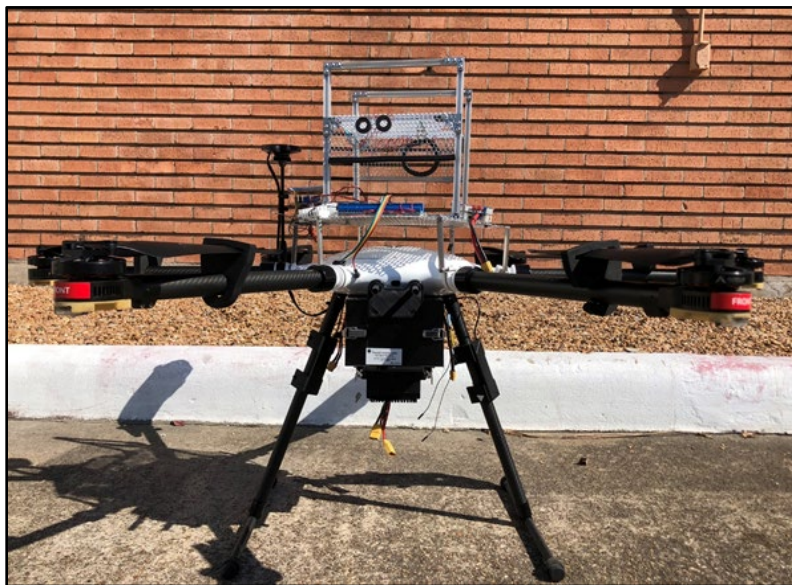
Figure 64: Chassis mounted to the top of the drone
