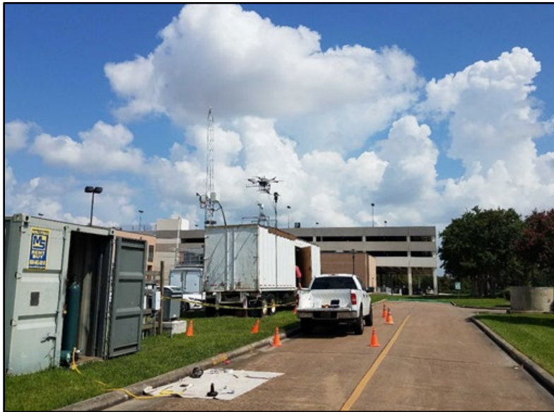
Figure 65: Drone in flight at the UH Launch Trailer (C1611) hovering near the inlet height for comparison of ozone measurement.
