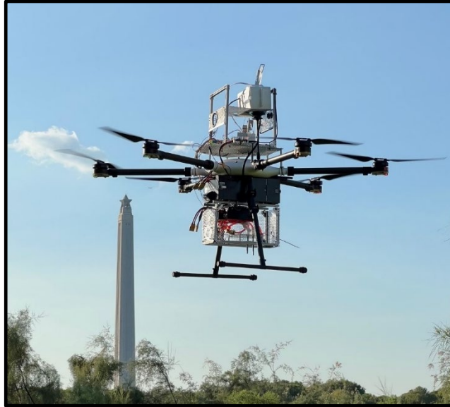
Figure 4: VOC sampler (below drone) mid-flight with ozone monitor (above drone) near the San Jacinto Monument (2022).
