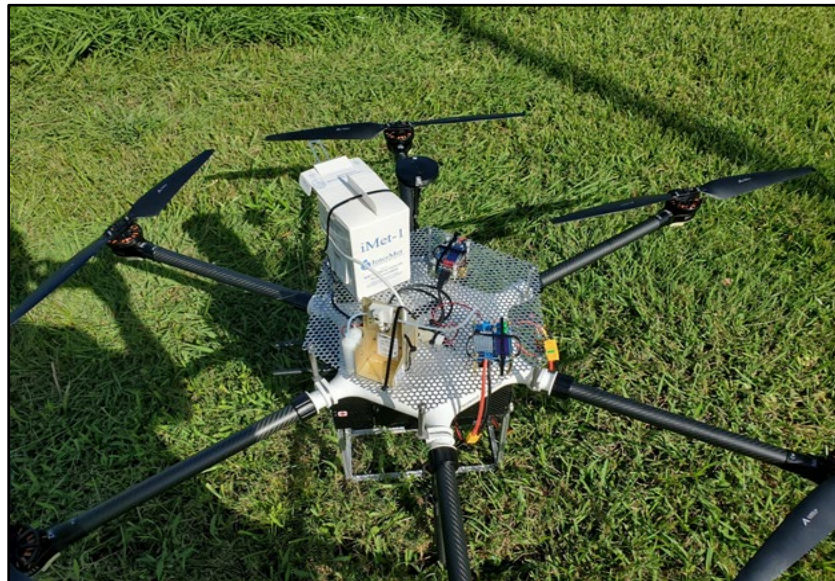
Figure 58: Ozone and meteorological sensors mounted to upper platform alongside voltage regulators.
