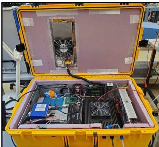
Figure 23: Instrumented weatherproof enclosure installed on the two commercial boats showing the 2B Tech O 3 monitor (blue box, bottom left), dual-sim cellular router (small blue box above 2B), backup battery (black box, center), zeroing cartridge (orange and clear, left rear), rugged industrial computer (black box with fan on top, right), high efficiency 24VDC power supply (silver box, far right). The rear panel of the chassis provides space for the LabJack U3 data card (red, center rear), thermoelectric temperature controller (black with green screen, rear behind computer), and circuit breaker for the thermoelectric cooler system (black button on silver tab, right of temperature controller). Space for mounting the NO 2 photocells is reserved on top of the O 3 analyzer, near the cellular router and will be installed for future campaigns.
