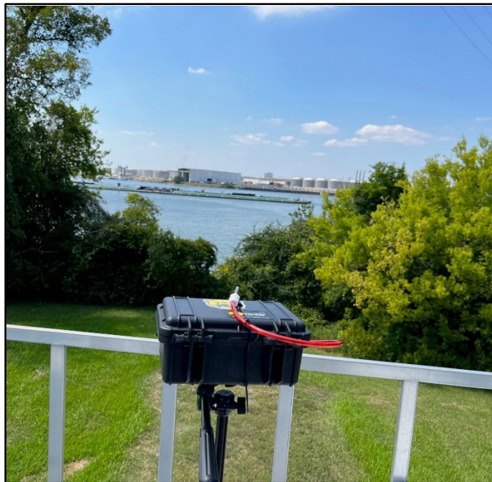
Figure 9: Custom-built sorbent tube sampler atop the MAQL2 at Battleground location
