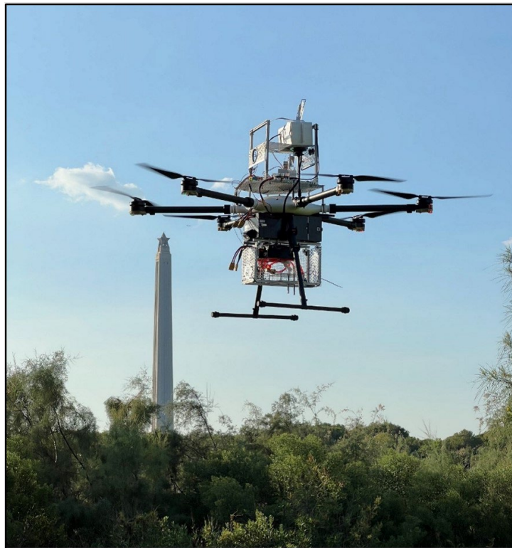
Figure 73: The Aurelia X6 Pro flying at San Jacinto Battleground Park. The primary payload is mounted on top and the VOC payload is mounted on the bottom.
