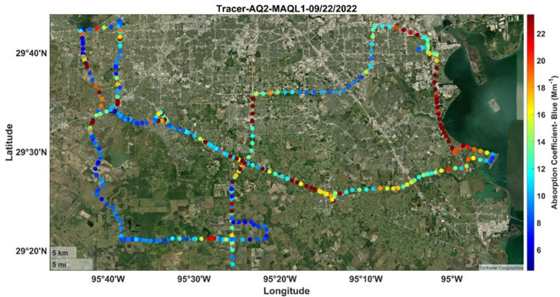
Figure 30: Spatial variability of the absorption coefficient of PM 5 at 365 nm (Blue) during the mobile measurement on 09/22/2022 in Houston.
