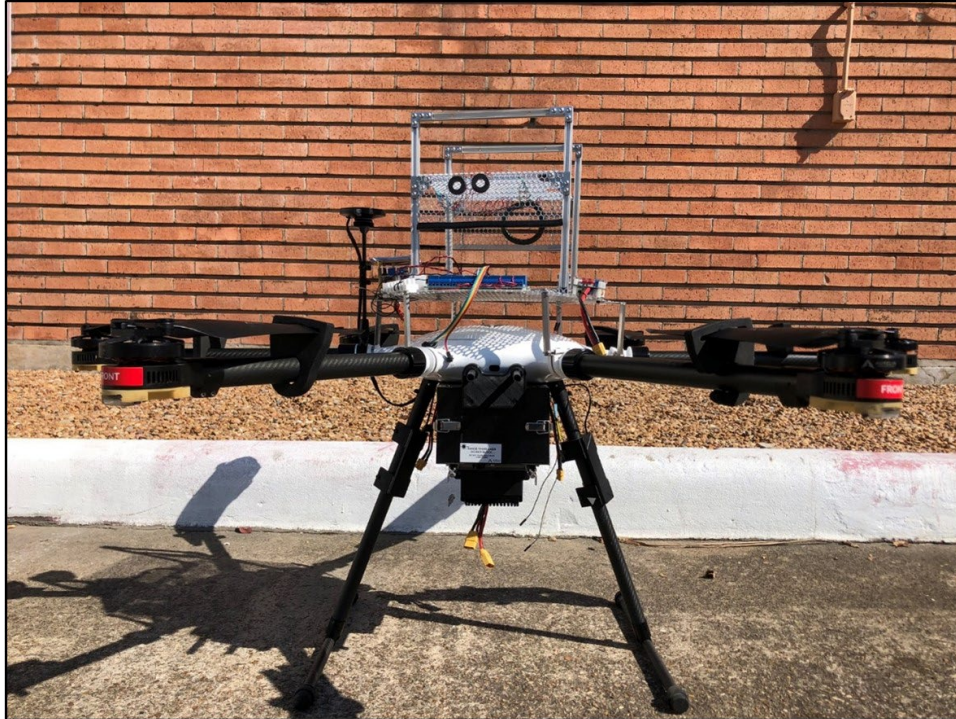
Figure 71: The Aurelia X6 Pro with the sensor chassis, electrical system components, and the upper platform mounted to the top of the drone.
