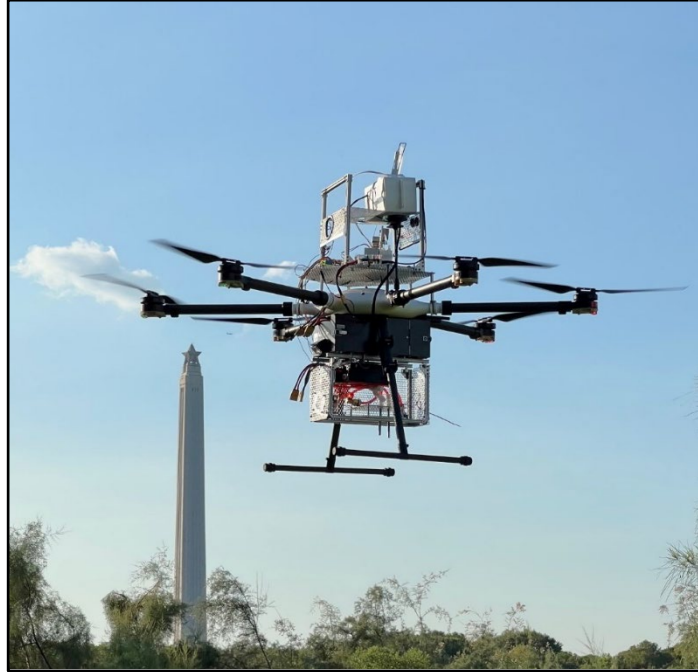
Figure 8: VOC sampler (below drone) mid-flight with ozone monitor (above drone) at the San Jacinto Monument
