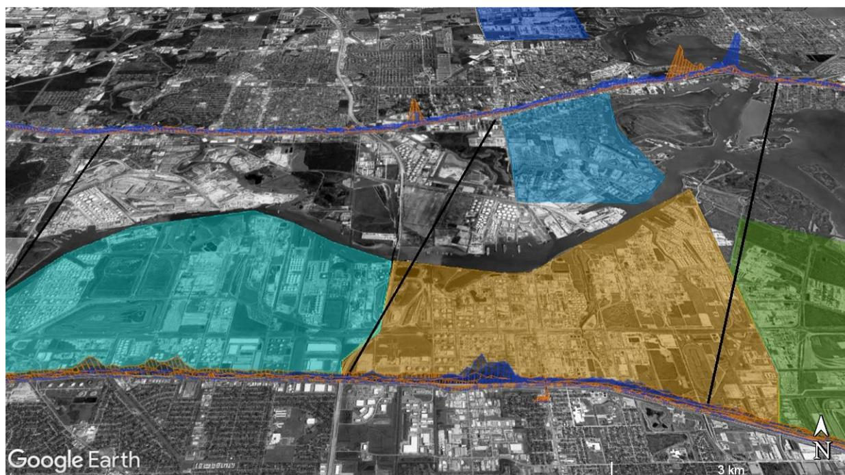
Figure 30 Example of concentration mapping data from MeDOAS showing benzene (blue, max 20 ppb) and Toluene (orange, max 18 ppb), in the Deer Park & Pasadena area and north of HSC, 09:39 - 17:57, 26 September. Winds from the east-northeast. Image mapped on Google Earth © 2022.
