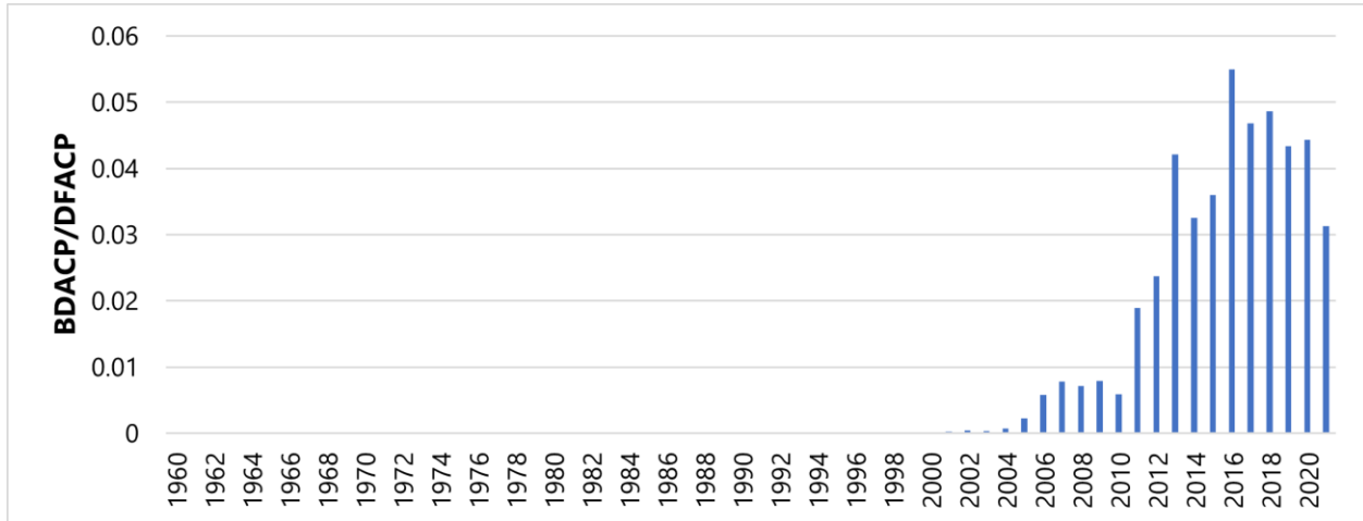
Figure 3-3. Annual Biodiesel Proportions of Transportation Sector Distillate Fuel Oil Sales from the SEDS Data.
