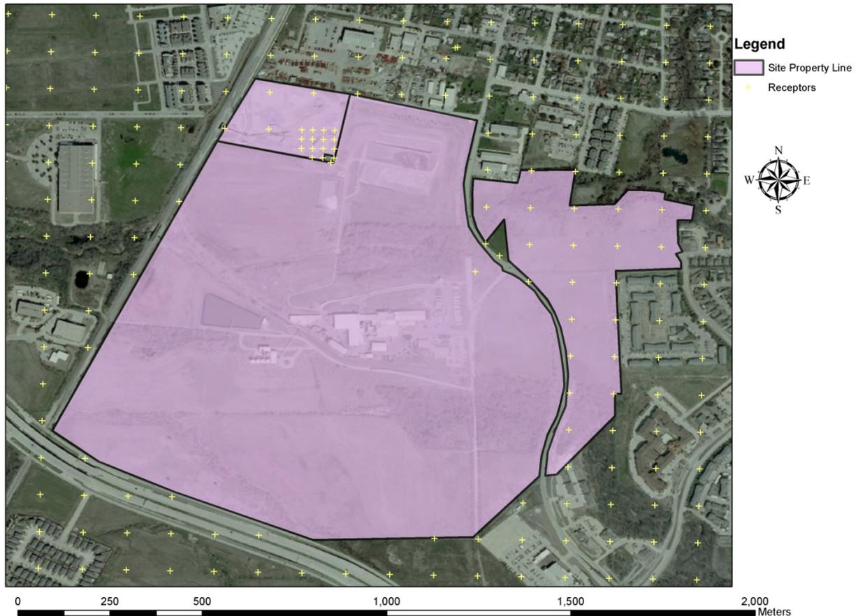
**Figure 3-3: Graphical Representation of Receptor Grid Showing Refined Grid**
