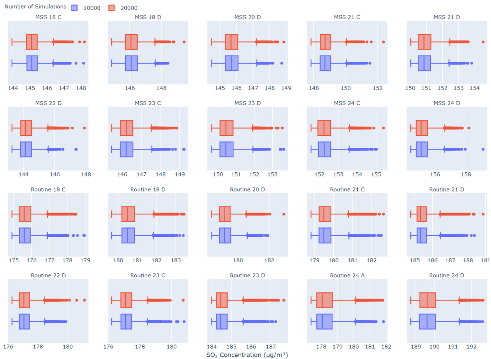
Figure 3. Comparison of Monte Carlo Runs with 10,000 and 20,000 Simulations for top 10 MSS and Routine Scenarios
