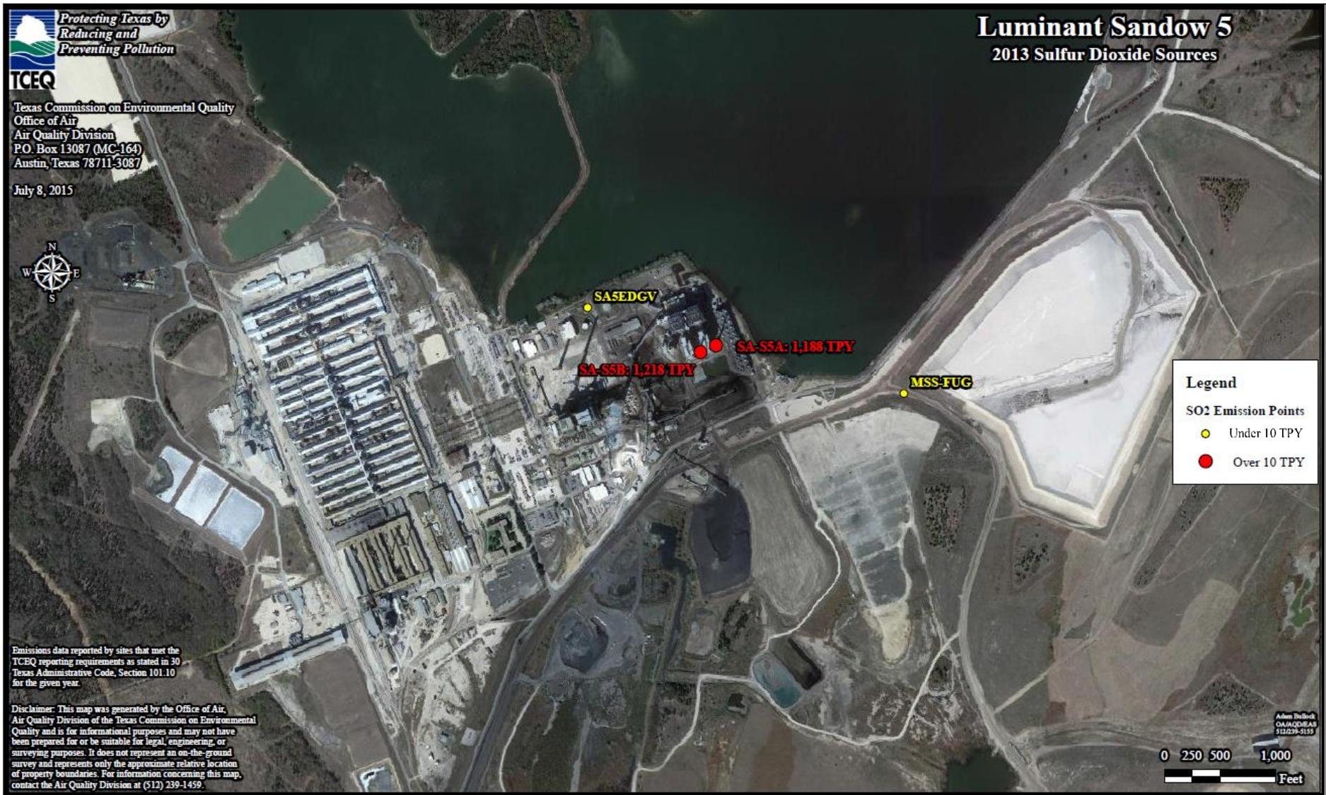
Figure 2: Sandow 5 Sulfur Dioxide (SO<sub>2</sub>) Stacks and Emissions, 2013
