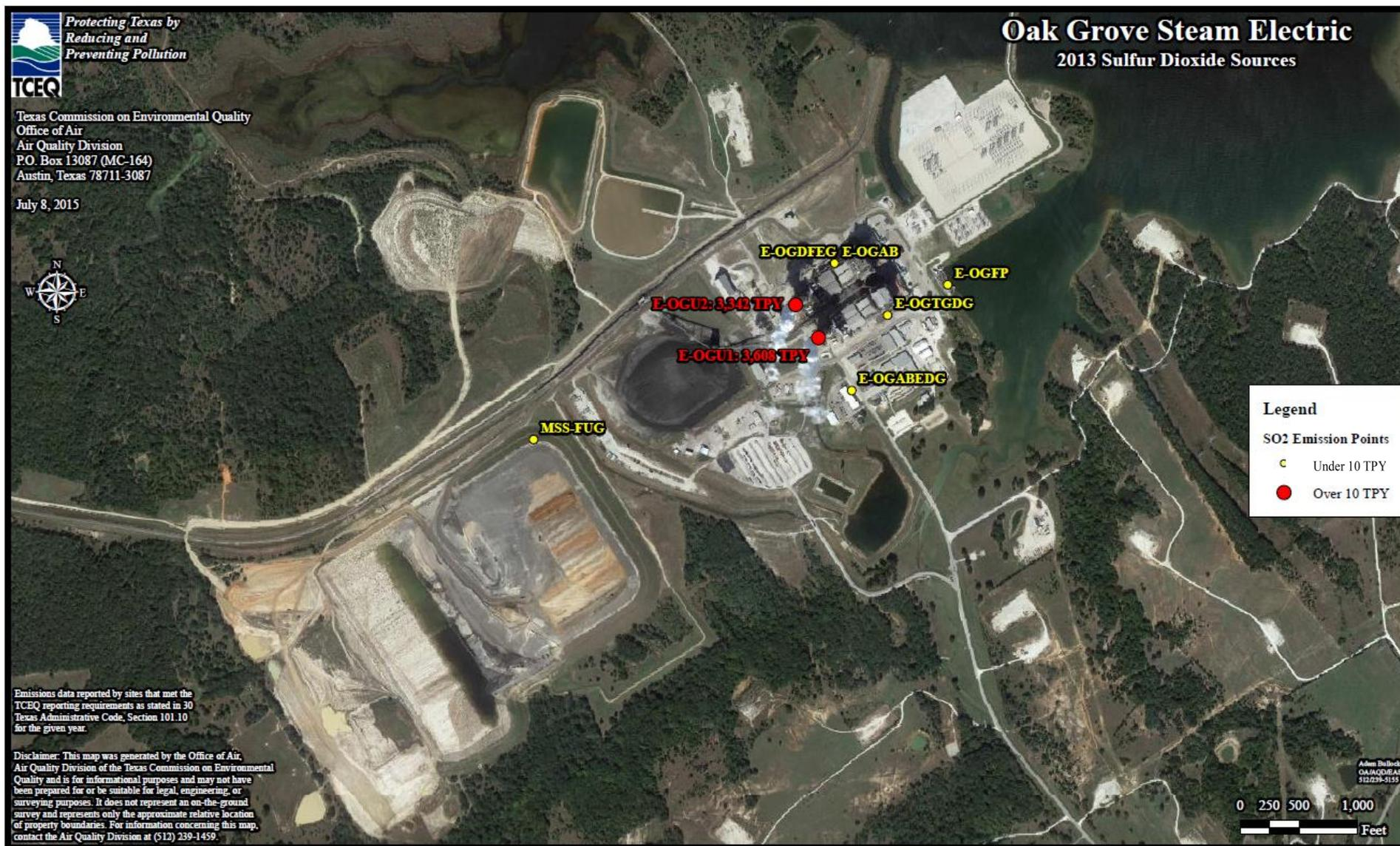
Figure 2: Oak Grove Sulfur Dioxide (SO<sub>2</sub>) Stacks and Emissions, 2013
