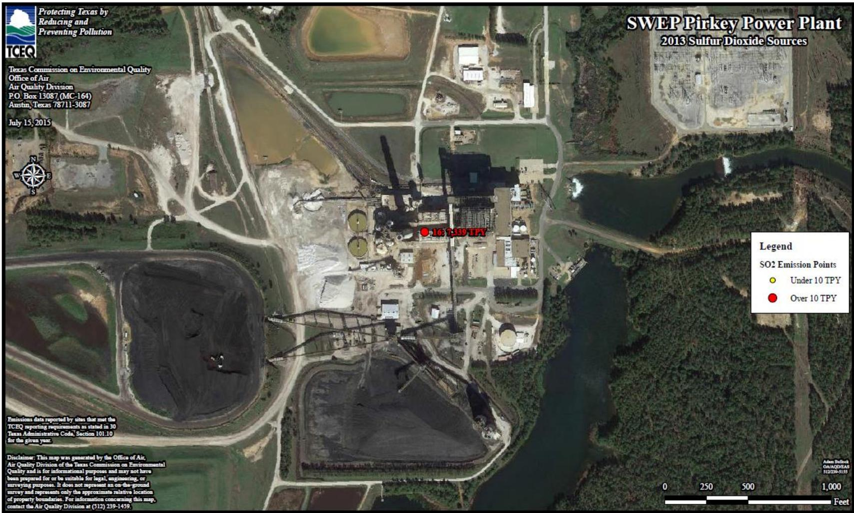
Figure 2: Pirkey Sulfur Dioxide Stacks and Emissions, 2013
