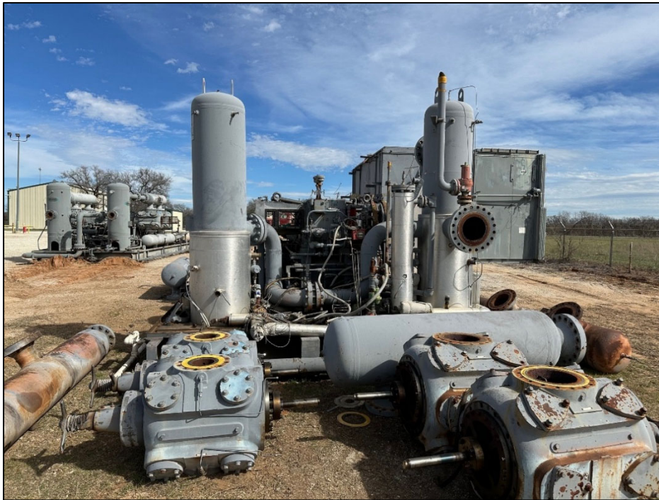
Both compressors shown (one in the foreground and one in the background), located at the Gordon during refurbishment by Colt's mechanical technicians
