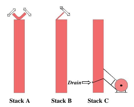
The examples on this page offer rain protection without obstructing air flow. The rain protection on stacks A and B is pushed up when the fan is on. Stack C is designed so that water drains out the side of the stack.
