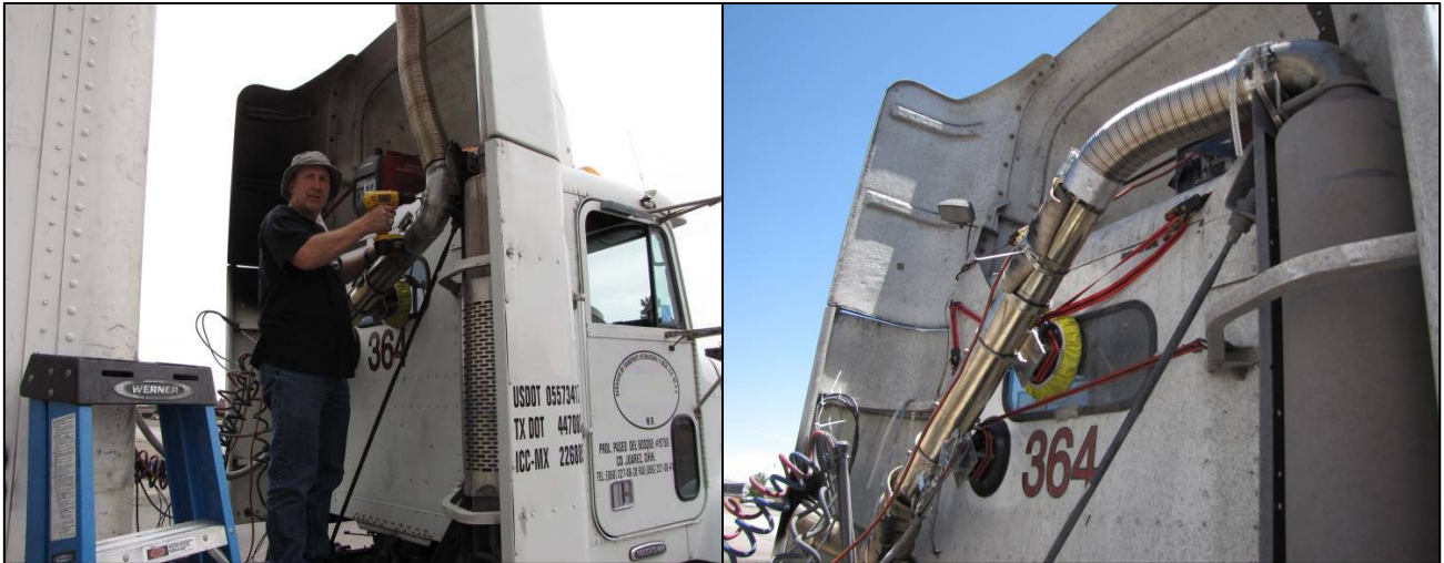
Figure 8. Photographs of Pre- and Post DOC installation (Left Photo Shows the Exhaust Flow Meter (EFM) Being Installed for the Baseline Test; Right Photo Shows the Same Vehicle with the DOC Installed).
