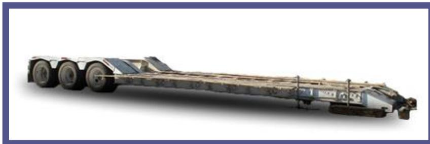
Loading capacity of 60 tons (132,277 pounds) and 3 axles.
