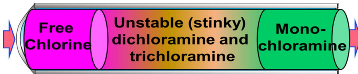
Figure 3. Unstable chloramines in a pipe at the boundary between water with a free chlorine residual and water with a monochloramine residual.
