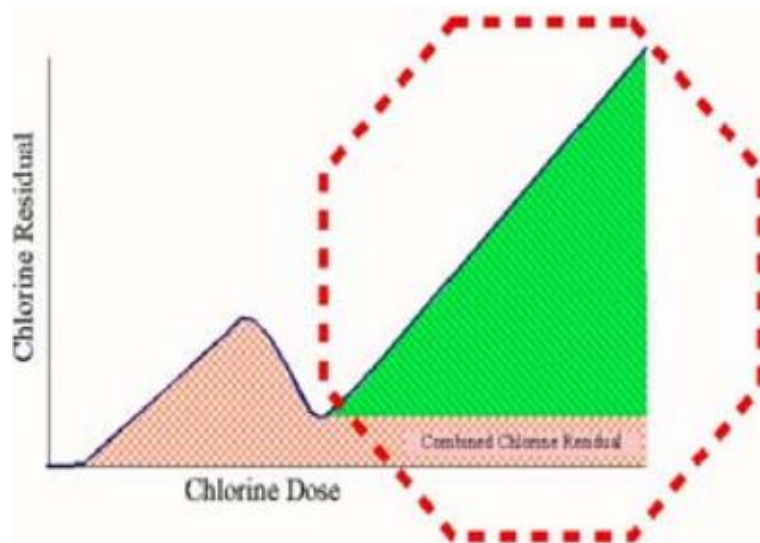
Figure 25. When you add free chlorine to water with very little ammonia, you are in Stage 6 of the Schulze breakpoint curve (Figure 4).
