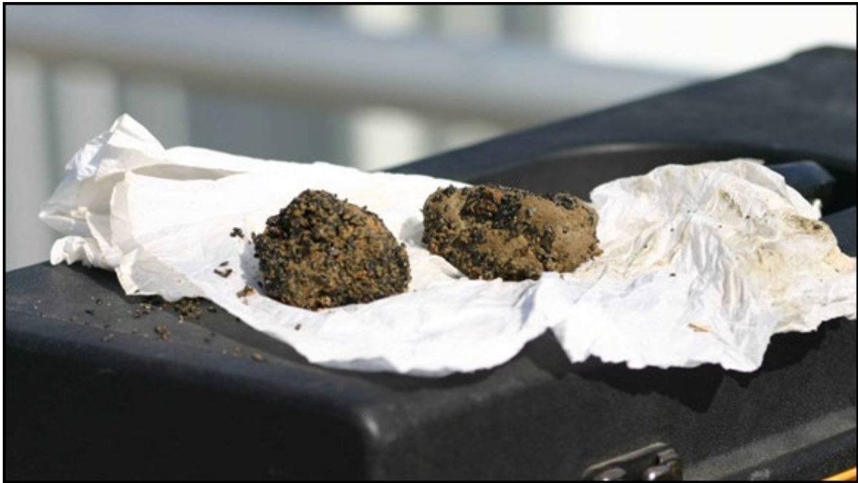
Figure 84: Mudballs from a Poorly Maintained Filter
