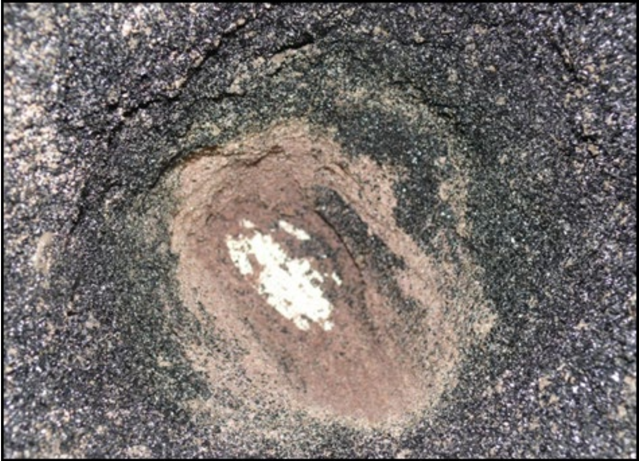
Figure 63: Photo of Poor Media Stratification
