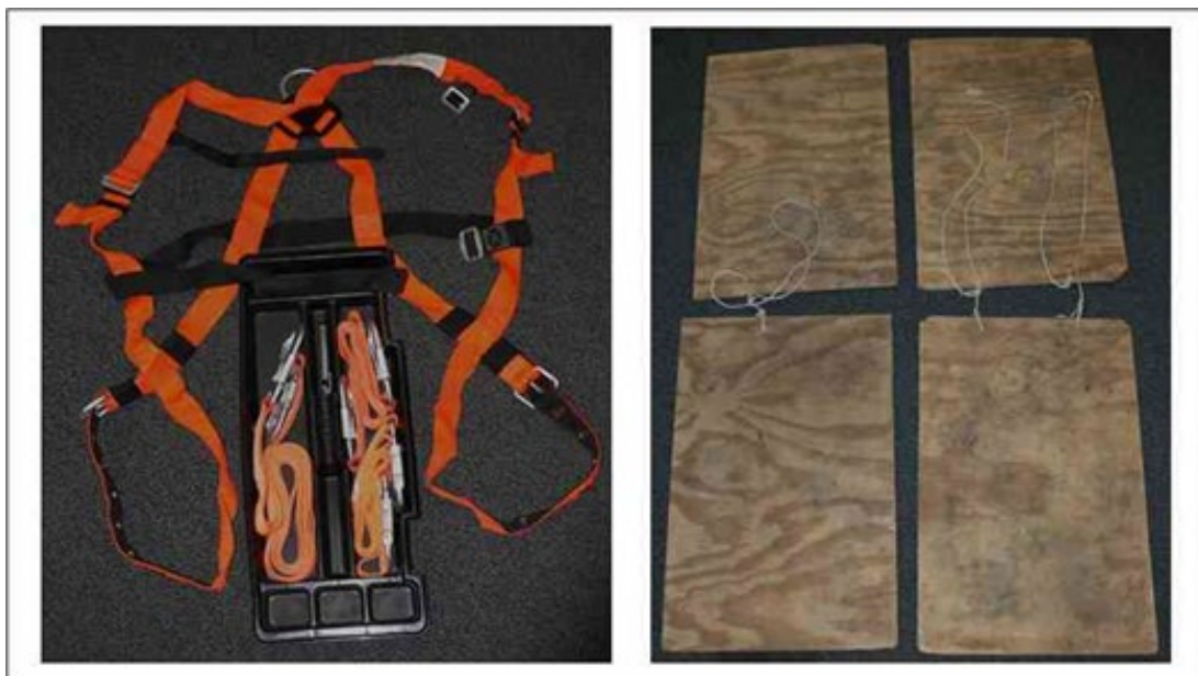
Figure 56: Safety Gear for Working In Filters
