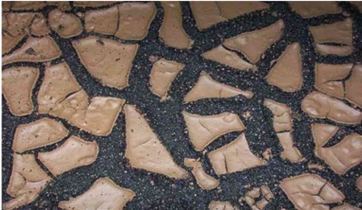
Figure 39: Surface Accumulations: These really aren't cracks... It's dried floc on top of a filter that was drained before backwashing.
