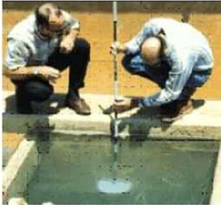
Figure 68: Two Engineers Measure Bed Expansion
