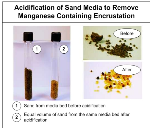
Figure 15: Removal of Manganese by Acidification
