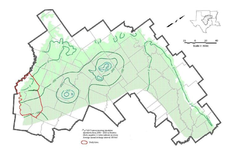
Figure 11. Simulated Water-level change from 2000 to 2030 for layer 7 (Hosston), Assuming Average Annual Recharge (Harden et al., 2004)
