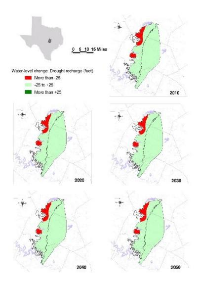
Figure 6. Simulated water-level changes 2010 through 2050, with drought-of-record recharge (Jones, 2003)
