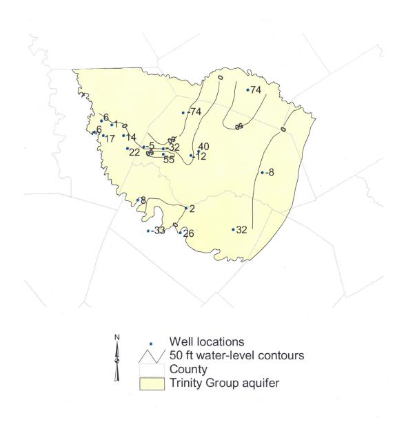
Figure 8. Water-level changes in the Trinity Group aquifers based on data collected 1987-1988 and data collected 1997-1998 (Ridgeway and Petrini, 1999)
