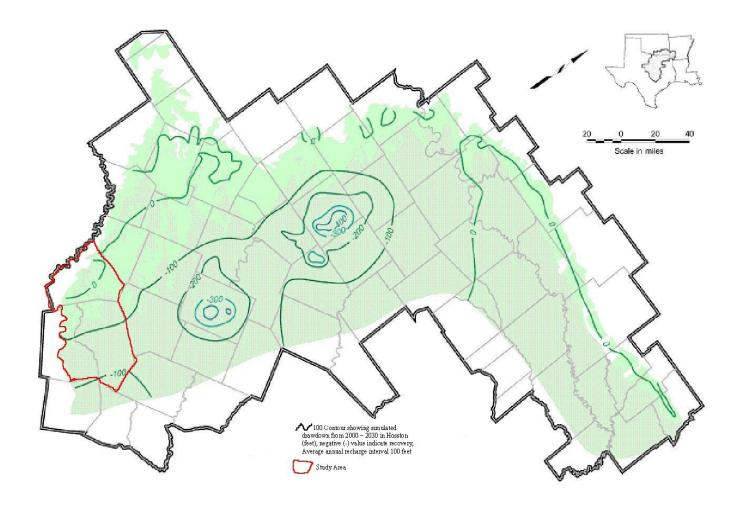
Figure 12. Simulated Water-level change from 2000 to 2030 for layer 7 (Hosston), Assuming Drought of record recharge distribution (Harden et al., 2004)
