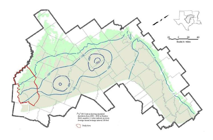
Figure 9. Simulated Water-level from 2000 to 2030 for layer 5 (Hensell), Assuming Average Recharge (Harden et al., 2004)
