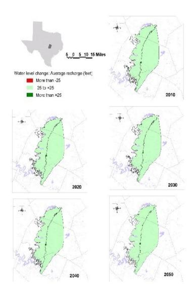
Figure 5. Simulated water-level changes 2010 through 2050, with average recharge. (Jones 2003)
