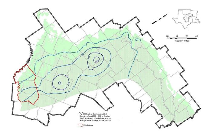
Figure 10. Simulated Water-level from 2000 to 2030 for layer 7 (Hensell), Assuming drought of record recharge distribution (Harden et al., 2004)
