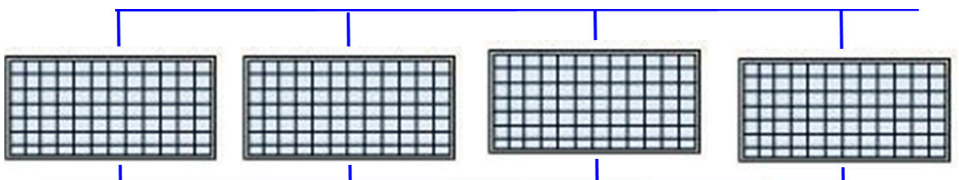
Figure 5. Solar voltaic panels in a parallel configuration [9].
