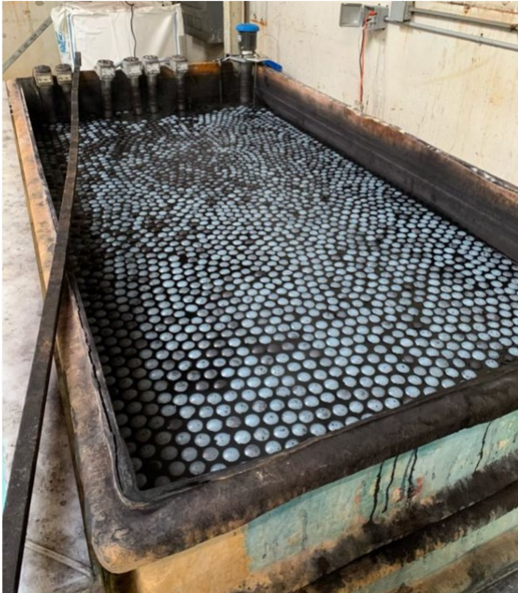
Polypropylene UFO's Installed in Black Dye Tank
