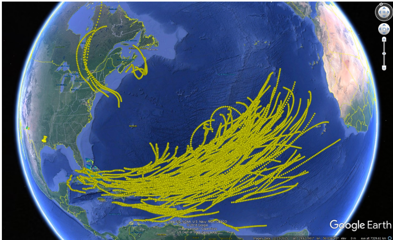
Figure 62 Ensemble of HYSPLIT back trajectories on suspected African dust impact dates, last 120 hours of 240 hour trajectories shown
