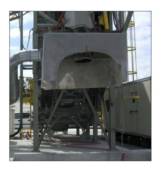
Three-sided enclosure with a flexible shroud hanging from above the truck (all plants and all locations) – improves control from 97.3% control to 99% control
